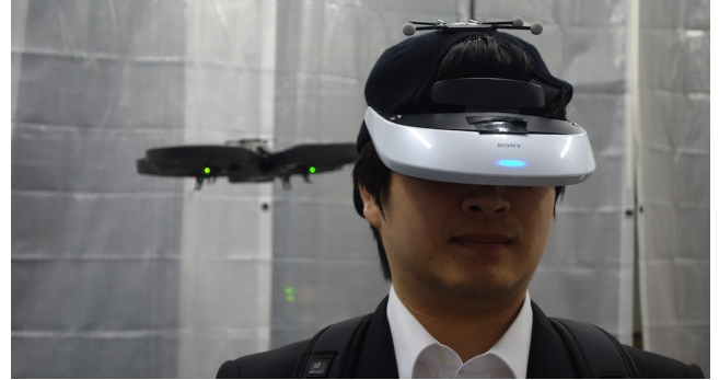
Figure 1: Flying Head is a telepresence system that remotely connects humans and unmanned aerial vehicles (UAVs). The system synchronizes the operator's head motions with the UAV's movement and it enables the operator to experience augmented abilities as if he or she became a flying robot.
